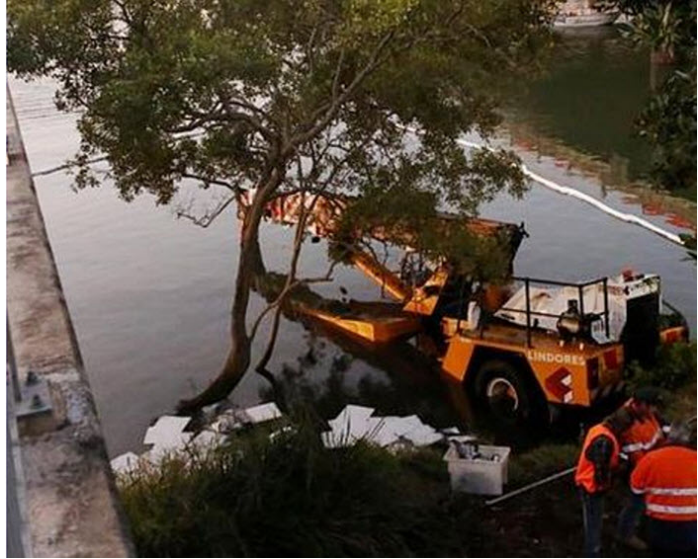
FIGURE 1: ARTICULATED NON-SLEWING CRANE CRASHED THROUGH A MOTORWAY BRIDGE
